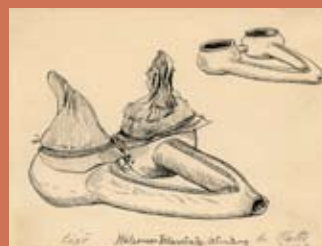
A wooden pair of bellows as used among the Kutti black smiths
